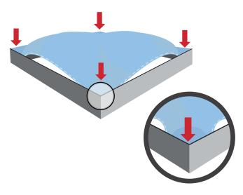
Important: Pivot the silicone edge behind the fabric, then insert into the channel.
