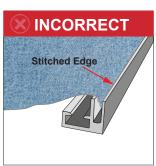
Step 2: From the center of each side insert graphic tucking the silicone edge into the channel on the front of the frame.
