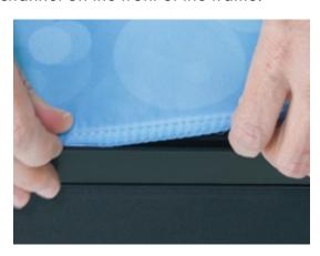
Step 3: Working your way from the center of each side insert graphic tucking the silicone edge into the channel on the front of the frame.
